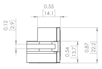
NOTE: BRAH ELECTRIC **COILS ARE A DIRECT** REPLACEMENT FOR GENERAL ELECTRIC, POWER BREAK 1, TYPE TR2, 100 Amp PLUG FOR 200 Amp CT SENSOR RATING, SUITABLE FOR USE WITH ALL TP, TC, THP, THC **EQUIPPED WITH** MICROVERSA TRIP RMS-9 SOLID STATE ELECTRONIC TRIP UNITS.
