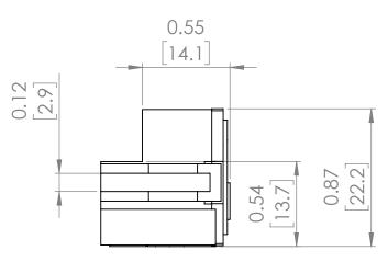
NOTE: BRAH ELECTRIC **COILS ARE A DIRECT** REPLACEMENT FOR GENERAL ELECTRIC, POWER BREAK 1, TYPE TR2, 2000 Amp PLUG FOR 2000 Amp CT SENSOR RATING, SUITABLE FOR USE WITH TP, TC, THP, THC EQUIPPED WITH MICROVERSA TRIP RMS-9 SOLID STATE ELECTRONIC TRIP UNITS.
