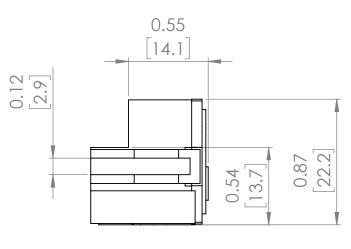
NOTE: BRAH ELECTRIC **COILS ARE A DIRECT** REPLACEMENT FOR GENERAL ELECTRIC, POWER BREAK 1, TYPE TR40, 1600 Amp PLUG FOR 4000 Amp CT SENSOR RATING, SUITABLE FOR USE WITH TP, TC, THP, THC, AKR100 **EQUIPPED WITH** MICROVERSA TRIP RMS-9 SOLID STATE ELECTRONIC TRIP UNITS.
