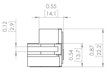
NOTE: BRAH ELECTRIC **COILS ARE A DIRECT** REPLACEMENT FOR GENERAL ELECTRIC, POWER BREAK 1, TYPE TR40, 4000 Amp PLUG FOR 4000 Amp CT SENSOR RATING, SUITABLE FOR USE WITH TP, TC, THP, THC, AKR100 **EQUIPPED WITH** MICROVERSA TRIP RMS-9 SOLID STATE ELECTRONIC TRIP UNITS.
