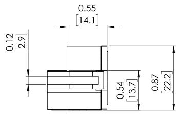
NOTE: BRAH ELECTRIC COILS ARE A DIRECT REPLACEMENT FOR GENERAL ELECTRIC, POWER BREAK 1, TYPE TR4, 200 Amp PLUG FOR 400 Amp CT SENSOR RATING, SUITABLE FOR USE WITH ALL TP, TC, THP, THC, AKR30H, AKR30S **EQUIPPED WITH** MICROVERSA TRIP RMS-9 SOLID STATE ELECTRONIC TRIP UNITS.
