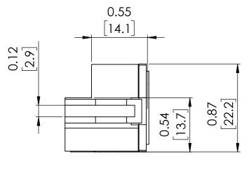
NOTE: BRAH ELECTRIC COILS ARE A DIRECT REPLACEMENT FOR GENERAL ELECTRIC, POWER BREAK 1, TYPE TR4, 300 Amp PLUG FOR 400 Amp CT SENSOR RATING, SUITABLE FOR USE WITH ALL TP, TC, THP, THC, AKR30H, AKR30S **EQUIPPED WITH** MICROVERSA TRIP RMS-9 SOLID STATE ELECTRONIC TRIP UNITS.
