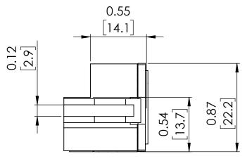
NOTE: BRAH ELECTRIC COILS ARE A DIRECT REPLACEMENT FOR GENERAL ELECTRIC, POWER BREAK 1, TYPE TR4, 400 Amp PLUG FOR 400 Amp CT SENSOR RATING, SUITABLE FOR USE WITH ALL TP, TC, THP, THC, AKR30H, AKR30S **EQUIPPED WITH** MICROVERSA TRIP RMS-9 SOLID STATE ELECTRONIC TRIP UNITS.
