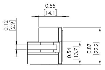
NOTE: BRAH ELECTRIC **COILS ARE A DIRECT** REPLACEMENT FOR GENERAL ELECTRIC, POWER BREAK 1, TYPE TR8,300 Amp PLUG FOR 800 Amp CT SENSOR RATING, SUITABLE FOR USE WITH ALL TP, TC, THP, THC, AKR30H, AKR30S, AKR50, AKR50H EQUIPPED WITH MICROVERSA TRIP **RMS-9 SOLID STATE** ELECTRONIC TRIP UNITS.
