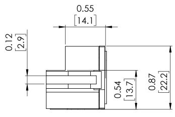
NOTE: BRAH ELECTRIC **COILS ARE A DIRECT** REPLACEMENT FOR GENERAL ELECTRIC, POWER BREAK 1, TYPE TR8,500 Amp PLUG FOR 800 Amp CT SENSOR RATING, SUITABLE FOR USE WITH ALL TP, TC, THP, THC, AKR30H, AKR30S, AKR50, AKR50H EQUIPPED WITH MICROVERSA TRIP **RMS-9 SOLID STATE** ELECTRONIC TRIP UNITS.
