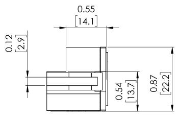
NOTE: BRAH ELECTRIC **COILS ARE A DIRECT** REPLACEMENT FOR GENERAL ELECTRIC, POWER BREAK 1, TYPE TR8,600 Amp PLUG FOR 800 Amp CT SENSOR RATING, SUITABLE FOR USE WITH ALL TP, TC, THP, THC, AKR30H, AKR30S, AKR50, AKR50H EQUIPPED WITH MICROVERSA TRIP **RMS-9 SOLID STATE** ELECTRONIC TRIP UNITS.
