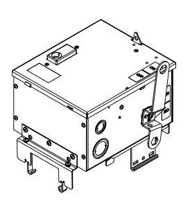
\* NOTE: BRAH Electric aftermarket SB361R, 30 amp, 600 volt, 3 phase, 3 wire, fusible style bus plug, type BEB / SB, UL Listed assembly, complete with UL Recognized internal switch and components
