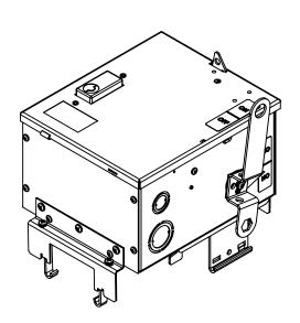
\* NOTE: BRAH Electric aftermarket direct SB362R, 60amp, 600volt, 3 phase, 3 wire, fusible style bus plug, type BEB / SB, UL Listed assembly, complete with UL Recognized internal switch and components.
