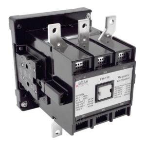
PART NUMBER - BEH-100: BRAH Electric, aftermarket direct replacement contactors for ABB EH-100, EH Series, type EH-100, 3P, 3PH, 120A, 600V, 40HP @ 240V, 75HP @ 480V, 100HP @ 600V, complete with 120V AC coil, 2 N/O - 2 N/C auxiliary contact, AC magnetic contactor, suitable for use with EH series motor control systems
