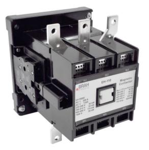
PART NUMBER - BEH-100-30-22: BRAH Electric, aftermarket direct replacement contactors for ABB EH-100, EH Series, type EH-100, 3P, 3PH, 120A, 600V, 40HP @ 240V, 75HP @ 480V, 100HP @ 600V, complete with 120V AC coil, 2 N/O - 2 N/C auxiliary contact, AC magnetic contactor
