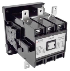
PART NUMBER - BEH-110: BRAH Electric, aftermarket direct replacement contactors for ABB EH-110, EH Series, type EH, 3P, 3PH, 120A, 600V, 40HP @ 240V, 75HP @ 480V, 100HP @ 600V, complete with 120V AC coil, 2 N/O - 2 N/C auxiliary contact, AC magnetic contactor, suitable for use with EH series motor control systems
