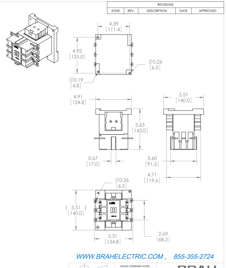
\* NOTE: THIS BRAH ELECTRIC CONTACTOR BEH-110-30-22 IS AN AFTERMARKET DIRECT REPLACEMENT FOR ABB EH-110-30-22, EH SERIES. SUITABLE FOR USE WITH EH SERIES MOTOR CONTROL SYSTEMS
