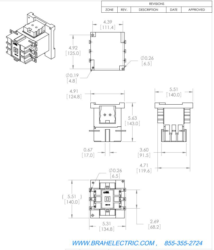
\* NOTE: THIS BRAH ELECTRIC CONTACTOR BEH-110-30-22AA IS AN AFTERMARKET DIRECT REPLACEMENT FOR ABB EH-110-30-22AA, EH SERIES. SUITABLE FOR USE WITH EH SERIES MOTOR CONTROL SYSTEMS
