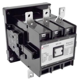
PART NUMBER - BEH-110-30-22AA: BRAH Electric, aftermarket direct replacement contactors for ABB EH-110-30-22AA, EH Series, type EH, 3P, 3PH, 120A, 600V, 40HP @ 240V, 75HP @ 480V, 100HP @ 600V, complete with 24V AC coil, 2 N/O - 2 N/C auxiliary contact, AC magnetic contactor, suitable for use with EH series motor control systems
