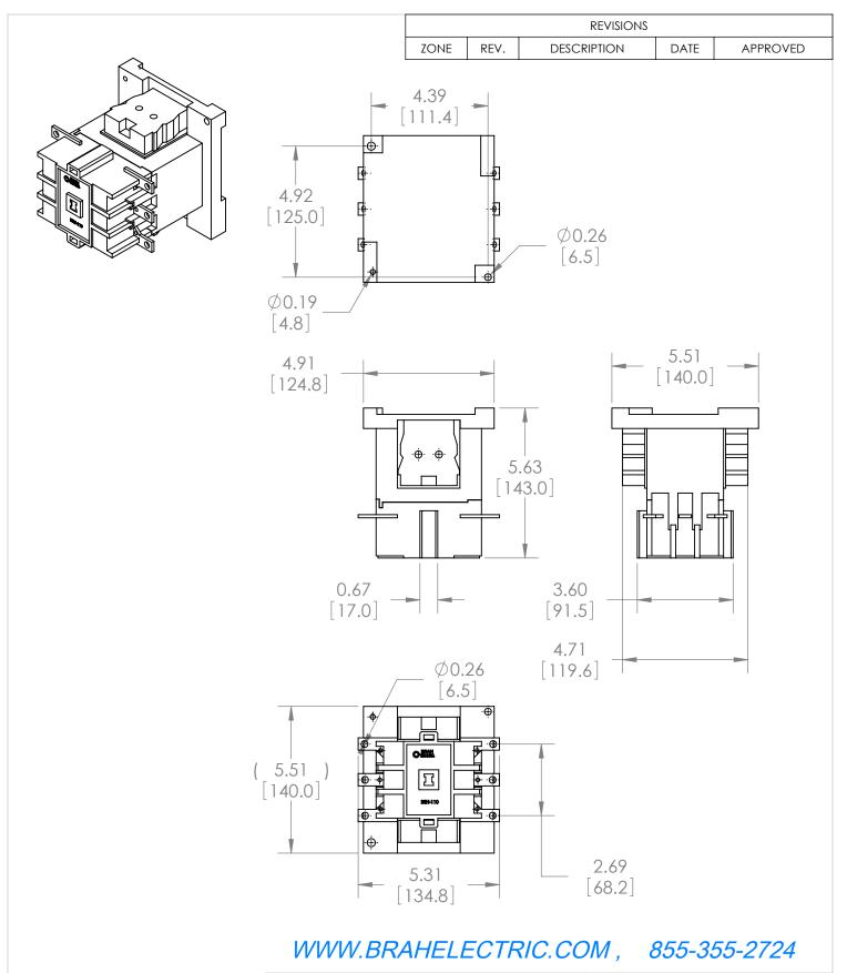
\* NOTE: THIS BRAH ELECTRIC CONTACTOR BEH-110-30-22AK IS AN AFTERMARKET DIRECT REPLACEMENT FOR ABB EH-110-30-22AK, EH SERIES. SUITABLE FOR USE WITH EH SERIES MOTOR CONTROL SYSTEMS
