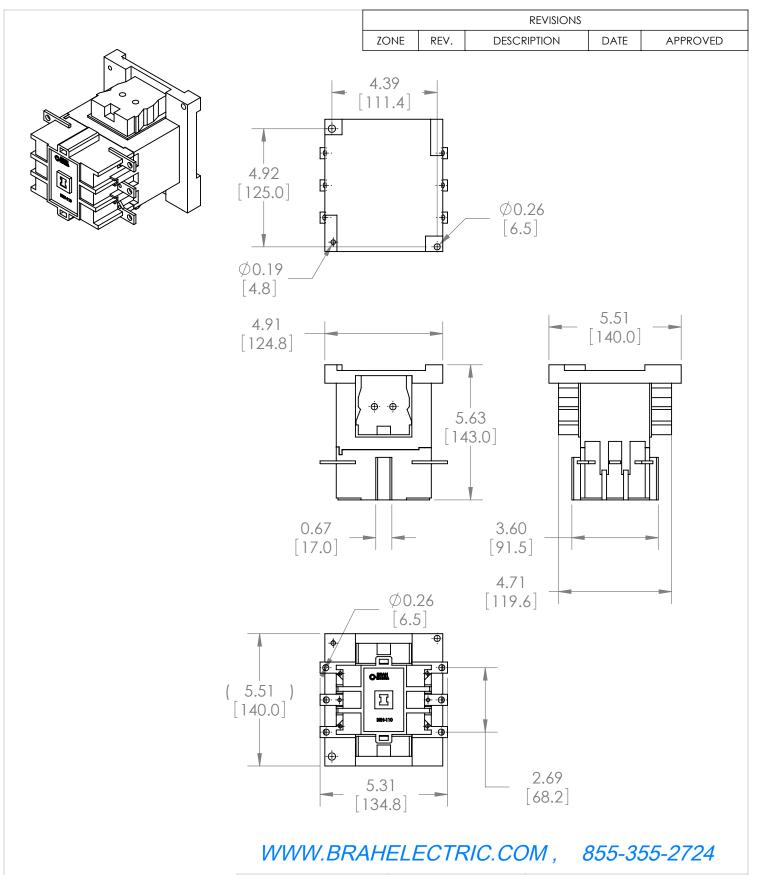
\* NOTE: THIS BRAH ELECTRIC CONTACTOR BEH-110-30-22AS IS AN AFTERMARKET DIRECT REPLACEMENT FOR ABB EH-110-30-22AS, EH SERIES. SUITABLE FOR USE WITH EH SERIES MOTOR CONTROL SYSTEMS
