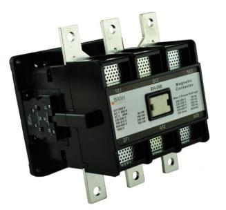
**PART NUMBER - BEH-260**: BRAH Electric, aftermarket direct replacement contactors for ABB EH-260, EH Series, type EH, 3P, 3PH, 260A, 600V, 100HP @ 240V, 200HP @ 480V, 250HP @ 600V, complete with 120V AC coil, 2 N/O - 2 N/C auxiliary contact, AC magnetic contactor, suitable for use with EH series motor control systems
