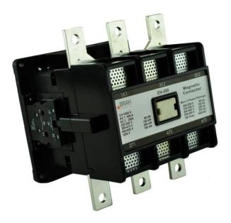
PART NUMBER - BEH-260-30-22AA: BRAH Electric, aftermarket direct replacement contactors for ABB EH-260-30-22AA, EH Series, type EH, 3P, 3PH, 260A, 600V, 100HP @ 240V, 200HP @ 480V, 250HP @ 600V, complete with 24V AC coil, 2 N/O - 2 N/C auxiliary contact, AC magnetic contactor, suitable for use with EH series motor control systems
