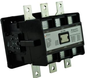
**PART NUMBER - BEH-300-30-22**: BRAH Electric, aftermarket direct replacement contactors for ABB EH-300-30-22, EH Series, type EH, 3P, 3PH, 305A, 600V, 100HP @ 240V, 250HP @ 480V, 250HP @ 600V, complete with 120V AC coil, 2 N/O - 2 N/C auxiliary contact, AC magnetic contactor, suitable for use with EH series motor control systems
