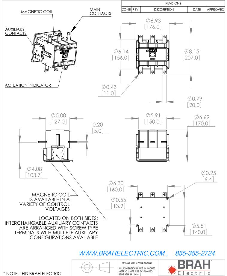
CONTACTOR BEH-300-30-22AS IS AN AFTERMARKET DIRECT REPLACEMENT FOR ABB EH-300-30-22AS, EH SERIES. SUITABLE FOR USE WITH EH SERIES MOTOR CONTROL SYSTEMS
