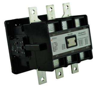
PART NUMBER - BEH-300-30-22AS: BRAH Electric, aftermarket direct replacement contactors for ABB EH-300-30-22AS, EH Series, type EH, 3P, 3PH, 305A, 600V, 100HP @ 240V, 250HP @ 480V, 250HP @ 600V, complete with 480V AC coil, 2 N/O - 2 N/C auxiliary contact, AC magnetic contactor, suitable for use with EH series motor control systems
