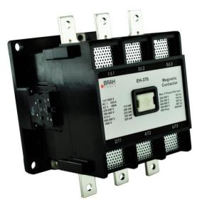
**PART NUMBER - BEH-370-30-22**: BRAH Electric, aftermarket direct replacement contactors for ABB EH-370-30-22, EH Series, type EH, 3P, 3PH, 400A, 600V, 140HP @ 240V, 300HP @ 480V, 400HP @ 600V, complete with 120V AC coil, 2 N/O - 2 N/C auxiliary contact, AC magnetic contactor, suitable for use with EH series motor control systems
