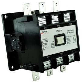
PART NUMBER - BEH-370-30-22AA: BRAH Electric, aftermarket direct replacement contactors for ABB EH-370-30-22AA, EH Series, type EH, 3P, 3PH, 400A, 600V, 140HP @ 240V, 300HP @ 480V, 400HP @ 600V, complete with 24V AC coil, 2 N/O - 2 N/C auxiliary contact, AC magnetic contactor, suitable for use with EH series motor control systems
