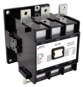
PART NUMBER - BEH-550: BRAH Electric, aftermarket direct replacement contactors for ABB EH-550, EH Series, type EH, 3P, 3PH, 550A, 600V, 200HP @ 240V, 400HP @ 480V, 500HP @ 600V, complete with 120V AC coil, 2 N/O - 2 N/C auxiliary contact, AC magnetic contactor, suitable for use with EH series motor control systems
