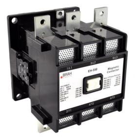
PART NUMBER - BEH-550-30-22: BRAH Electric, aftermarket direct replacement contactors for ABB EH-550-30-22, EH Series, type EH, 3P, 3PH, 550A, 600V, 200HP @ 240V, 400HP @ 480V, 500HP @ 600V, complete with 120V AC coil, 2 N/O - 2 N/C auxiliary contact, AC magnetic contactor, suitable for use with EH series motor control systems
