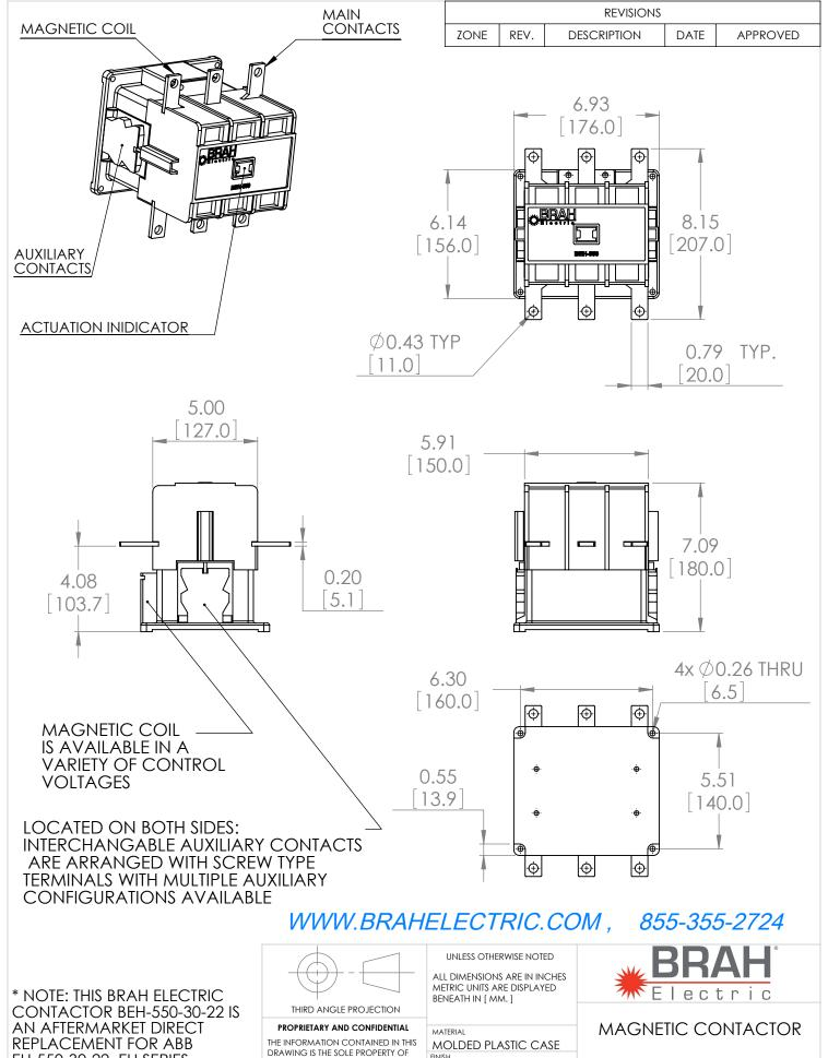
EH-550-30-22, EH SERIES. SUITABLE FOR USE WITH EH SERIES MOTOR CONTROL SYSTEMS
