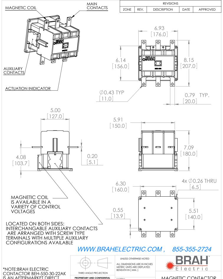
IS AN AFTERMARKET DIRECT REPLACEMENT FOR ABB EH-550-30-22AK, EH SERIES. SUITABLE FOR USE WITH EH SERIES MOTOR CONTROL SYSTEMS
