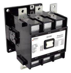
PART NUMBER - BEH-550-30-22AK: BRAH Electric, aftermarket direct replacement contactors for ABB EH-550-30-22AK, EH Series, type EH, 3P, 3PH, 550A, 600V, 200HP @ 240V, 400HP @ 480V, 500HP @ 600V, complete with 240V AC coil, 2 N/O - 2 N/C auxiliary contact, AC magnetic contactor, suitable for use with EH series motor control systems
