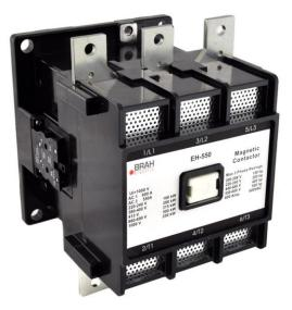
**PART NUMBER - BEH-550-30-22AS:** BRAH Electric, aftermarket direct replacement contactors for ABB EH-550-30-22AS, EH Series, type EH, 3P, 3PH, 550A, 600V, 200HP @ 240V, 400HP @ 480V, 500HP @ 600V, complete with 480V AC coil, 2 N/O - 2 N/C auxiliary contact, AC magnetic contactor, suitable for use with EH series motor control systems
