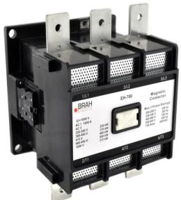
**PART NUMBER - BEH-700**: BRAH Electric, aftermarket direct replacement contactors for ABB EH-700, EH Series, type EH, 3P, 3PH, 700A, 600V, 300HP @ 240V, 550HP @ 480V, 650HP @ 600V, complete with 120V AC coil, 2 N/O - 2 N/C auxiliary contact, AC magnetic contactor, suitable for use with EH series motor control systems
