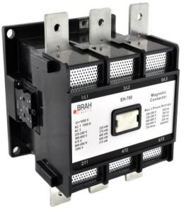
aftermarket direct replacement contactors for ABB EH-700-30-22, EH Series, type EH, 3P, 3PH, 700A, 600V, 300HP @ 240V, 550HP @ 480V, 650HP @ 600V, complete with 120V AC coil, 2 N/O - 2 N/C auxiliary contact, AC magnetic contactor, suitable for use with EH series motor control systems
