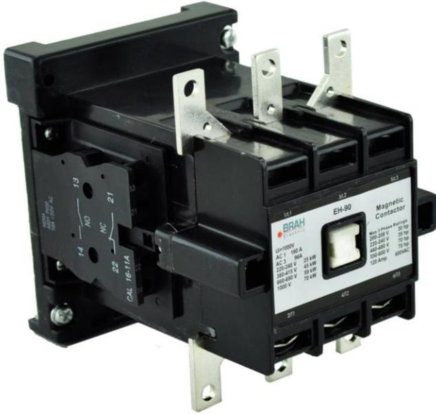
**PART NUMBER - BEH-80:** BRAH Electric, aftermarket direct replacement contactors for ABB EH-80, EH Series, type EH, 3P, 3PH, 80A, 600V, 35HP @ 240V, 70HP @ 480V, 70HP @ 600V, complete with 120V AC coil, 2 N/O - 2 N/C auxiliary contacts, AC magnetic contactor, suitable for use with EH series motor control systems
