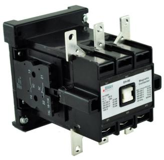
PART NUMBER - BEH-80-30-22: BRAH Electric, aftermarket direct replacement contactors for EH-80-30-22, EH Series, type EH, 3P, 3PH, 80A, 600V, 35HP @ 240V, 70HP @ 480V, 70HP @ 600V, complete with 120V AC coil, 2 N/O - 2 N/C auxiliary contacts, AC magnetic contactor, suitable for use with EH series motor control systems
