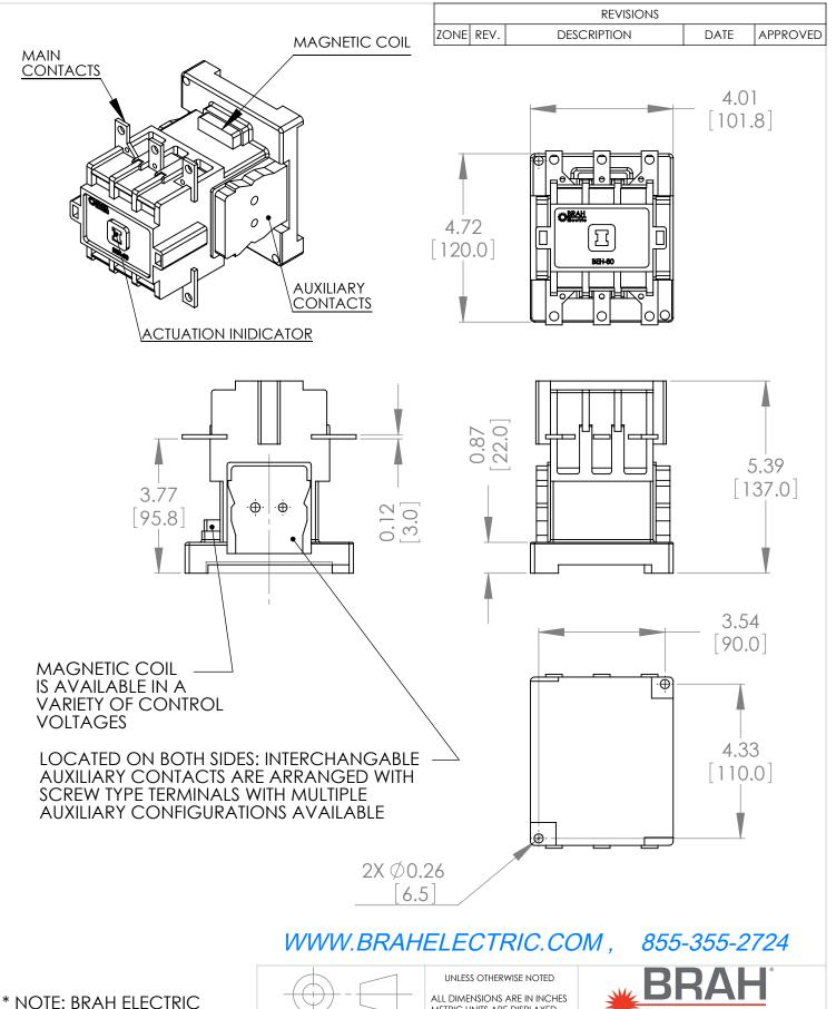
CONTACTOR BEH-80-30-22 IS AN AFTERMARKET DIRECT REPLACMENT FOR ABB EH-80-30-22, EH SERIES. SUITABLE FOR USE WITH EH SERIES MOTOR CONTROL SYSTEMS
