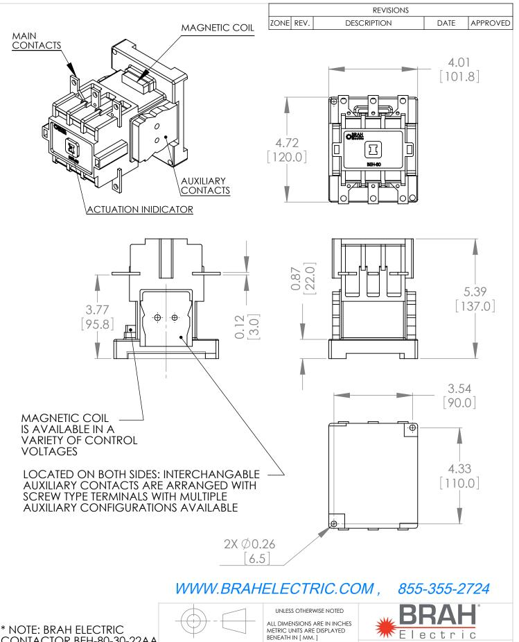
CONTACTOR BEH-80-30-22AA IS AN AFTERMARKET DIRECT REPLACMENT FOR ABB EH-80-30-22AA, EH SERIES. SUITABLE FOR USE WITH EH SERIES MOTOR CONTROL SYSTEMS
