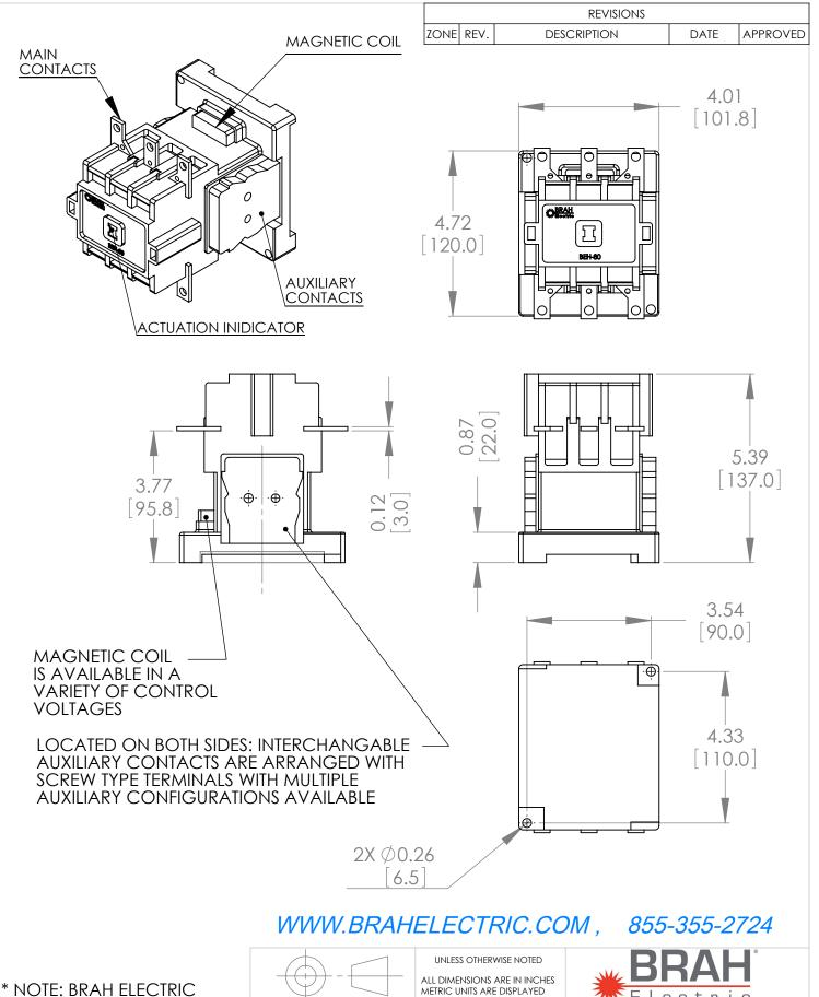
CONTACTOR BEH-80-30-22AS IS AN AFTERMARKET DIRECT REPLACMENT FOR ABB EH-80-30-22AS, EH SERIES. SUITABLE FOR USE WITH EH SERIES MOTOR CONTROL SYSTEMS
