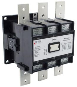
PART NUMBER - BEH-800-30-22AS: BRAH Electric, aftermarket direct replacement contactors for ABB EH-800-30-22AS, EH Series, type EH, 3P, 3PH, 750A, 600V, 300HP @ 240V, 600HP @ 480V, 700HP @ 600V, complete with 480V AC coil, 2 N/O - 2 N/C auxiliary contact, AC magnetic contactor, suitable for use with EH series motor control systems
