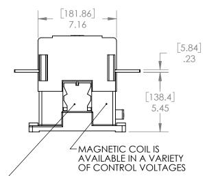
LOCATED ON BOTH SIDES. INTERCHANGEABLE AUXILIARY CONTACTS ARE ARRANGED WITH SCREW TYPE TERMINALS WITH MULTIPLE AUXILIARY CONFIGURATIONS AVAILABLE.
