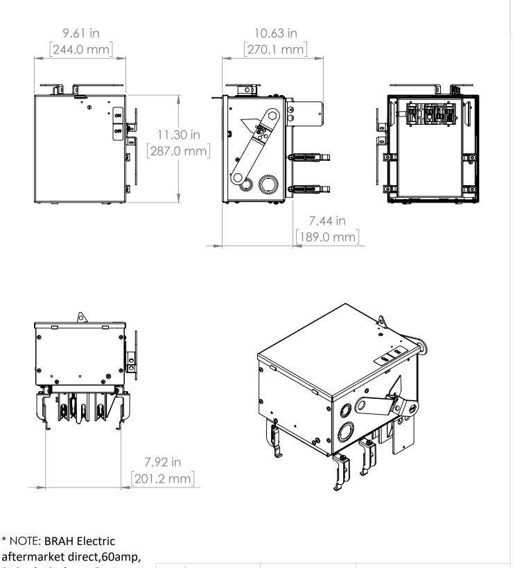
aftermarket direct,60amp, 240volt, 3 phase, 3 wire, fusible style bus plug, type BEK / FVK, suitable for use with OEM General Electric Flux-A-Plug series industrial Busway System.
