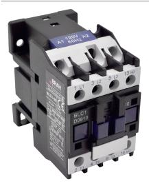
PART NUMBER – BLC1D0910-G7: BRAH Electric, aftermarket direct replacement contactors for Telemecanique LC1D0910-G7, TeSys D Series, type LC1D, 3P, 3PH, 25A, 600V, complete with 110/120V AC coil voltage max 5 hp, 1 N/O auxiliary contact, AC magnetic contactor, suitable for use with LC1-D series motor control systems.
