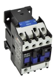
PART NUMBER – BLC1D1210: BRAH Electric, aftermarket direct replacement contactors for Telemecanique LC1D1210, TeSys D Series, type LC1D, 3P, 3PH, 25A, 600V, complete with 110/120V AC coil voltage max 7.5 hp, 1 N/O auxiliary contact, AC magnetic contactor, suitable for use with LC1-D series motor control systems.
