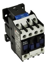
**PART NUMBER – BLC1D1810-B6**: BRAH Electric, aftermarket direct replacement contactors for Telemecanique LC1D1810-B6, TeSys D Series, type LC1D, 3P, 3PH, 32A, 600V, complete with 24V AC coil voltage max 10 hp, 1 N/O auxiliary contact, AC magnetic contactor, suitable for use with LC1-D series motor control systems.
