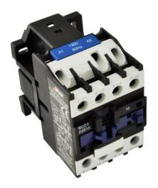
PART NUMBER – BLC1D2510-G7: BRAH Electric, aftermarket direct replacement contactors for Telemecanique LC1D2510-G7, TeSys D Series, type LC1D, 3P, 3PH, 40A, 600V, 7.5HP @ 240V, 15HP @ 480V, 20HP @ 600V, complete with 110/120V AC 50/60Hz coil, and 1 N/O auxiliary contact, AC magnetic contactor, suitable for use with LC1-D series motor control systems
