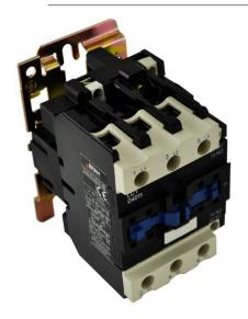
PART NUMBER – BLC1D4011: BRAH Electric, aftermarket direct replacement contactors for Telemecanique LC1D4011, TeSys D Series, type LC1D, 3P, 3PH, 60A, 600V, 10HP @ 240V, 30HP @ 480V, 30HP @ 600V, complete with 110/120V AC coil, and 1 N/O - 1 N/C auxiliary contact, AC magnetic contactor, suitable for use with LC1-D series motor control systems
