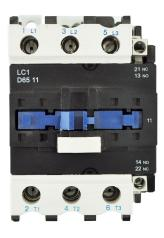
PART NUMBER – BLC1D6511: BRAH Electric, aftermarket direct replacement contactors for Telemecanique LC1D6511, TeSys D Series, type LC1D, 3P, 3PH, 80A, 600V, complete with 110/120V AC coil voltage max 40 hp, 1 N/O - 1 N/C auxiliary contact, AC magnetic contactor, suitable for use with LC1-D series motor control systems.
