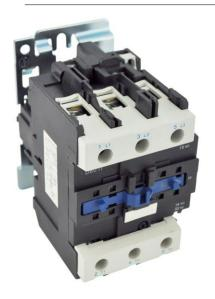
PART NUMBER –BLC1D8011-B7: BRAH Electric, aftermarket direct replacement contactors for Telemecanique LC1D8011-B7, TeSys D Series, type LC1D, 3P, 3PH, 125A, 600V, 30HP @ 240V, 60HP @ 480V, 60HP @ 600V, complete with 24V AC 50/60Hz coil, and 1 N/O - 1 N/C auxiliary contact, AC magnetic contactor, suitable for use with LC1-D series motor control systems
