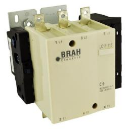
MAGNETIC CONTACTOR PART NO. BLC1F115 <u>PART NUMBER – BLC1F115</u>: BRAH Electric, aftermarket direct replacement contactors for Telemecanique LC1F115, TeSys F Series, type LC1F, 3P, 3PH, 115A, 600V, 40HP @ 240V, 75HP @ 480V, 100HP @ 600V, complete with 120V AC coil, AC magnetic contactor, suitable for use with LC1-F series motor control systems
