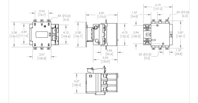
\*NOTE: BRAH ELECTRIC CONTACTOR BLC1F185 IS AN AFTERMARKET DIRECT REPLACMENT FOR LC1F185, LC1-F SERIES. SUITABLE FOR USE WITH LC1-F SERIES MOTOR CONTROL SYSTEMS
