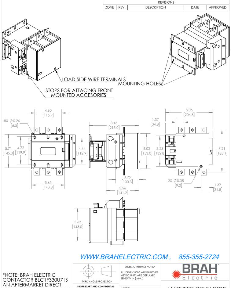
REPLACMENT FOR LC1F330U7, LC1-F SERIES. SUITABLE FOR USE WITH LC1-F SERIES MOTOR CONTROL SYSTEMS
