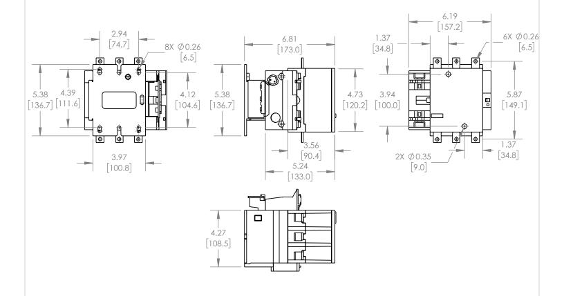
\*NOTE: BRAH ELECTRIC CONTACTOR BLC1F400 IS AN AFTERMARKET DIRECT REPLACMENT FOR LC1F400, LC1-F SERIES. SUITABLE FOR USE WITH LC1-F SERIES MOTOR CONTROL SYSTEMS
