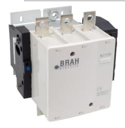
PART NUMBER – BLC1F400: BRAH Electric, aftermarket direct replacement contactors for Telemecanique LC1F400, TeSys F Series, type LC1F, 3P, 3PH, 500A, 600V, 125HP @ 240V, 250HP @ 480V, 300HP @ 600V, complete with 120V AC coil, AC magnetic contactor, AC magnetic contactor, suitable for use with LC1-F series motor control systems
