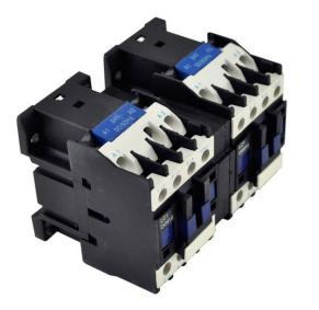
PART NUMBER – BLC2D0910: BRAH Electric, aftermarket direct replacement reversing contactors for Telemecanique LC2D0910, TeSys D Series, type LC2D, 3P, 3PH, 25A, 600V, 0.5-2HP @ 240V, 0.5-5HP @ 480V, 7.5HP @ 600V, both complete with 110/120V AC coil, 1 N/O auxiliary contact, AC magnetic contactor, suitable for use with LC2-D series motor control systems
