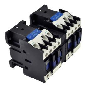
**PART NUMBER – BLC2D0910-M6**: BRAH Electric, aftermarket direct replacement reversing contactors for Telemecanique LC2D0910-M6, TeSys D Series, type LC2D, 3P, 3PH, 25A, 600V, 0.5-2HP @ 240V, 0.5-5HP @ 480V, 7.5HP @ 600V, both complete with 220V 60Hz AC coil, 1 N/O auxiliary contact, AC magnetic contactor, suitable for use with LC2-D series motor control systems
